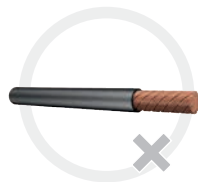
Excessively twisted individual wires
