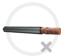
Remains of the conductor insulation on the stripped conductor
