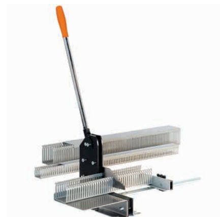
Wire channel cutter for manual operation in cutting wiring channels and covers up to 125 mm wide and a wall thickness of 2.5 mm. Not suitable for plastics reinforced by fillers plastics.
